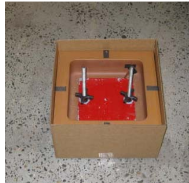
Block with Static Load on Corners
